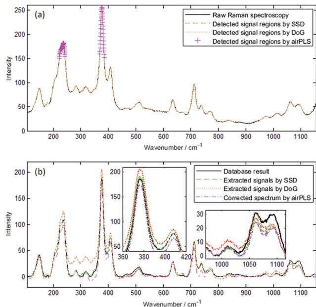
Fig. 10 Real fluoriddicoatite spectrum: (a) signal region detection and (b) signal extraction.
