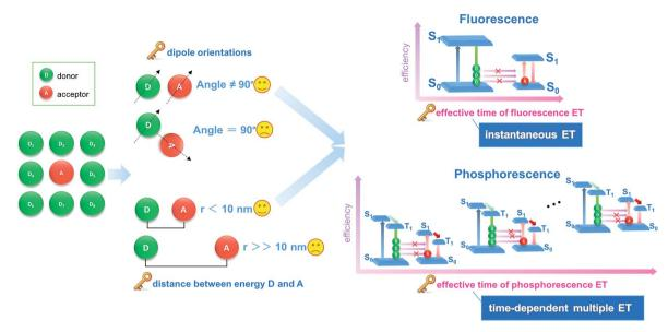
Fig. 1 Schematic illustration of different energy transfer (ET) processes showing how phosphorescence energy transfer (PET) leads to more efficiency than conventional fluorescence energy transfer (FET).
