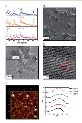
Fig. 3 Structure and morphology of LDHs nanosheets. (a) XRD patterns for PA/LDH, IPA/LDH and TPA/LDH. (b) SEM image for IPA/LDH. (c) The TEM image and (d) high-resolution TEM of IPA/LDH (inset image in c shows an individual IPA/LDH nanosheet). (e) AFM image and the height curves for IPA/LDH.
