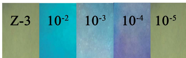
Fig. 5 Photographs of test strips (the concentration of Hg 2+ is 0 M, 10^{-1} \text{ M} , 10^{-2} \text{ M} , 10^{-3} \text{ M} , 10^{-4} \text{ M} , 10^{-5} \text{ M} , both under an UV lamp at 365 nm).
