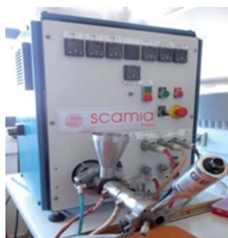
Fig. 7 Representation of a single-screw extruder.
