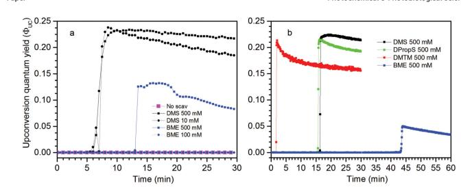
Fig. 3 The measured  $\phi_{UC}$  in filled screw-cap vials during continuous irradiation at 532 nm. (a) High concentration TTA-UC system ([PdOEP] = 16  $\mu$ M and [DPA] = 500  $\mu$ M) and (b) lower concentration system ([PdOEP] = 5  $\mu$ M and [DPA] = 100  $\mu$ M).
