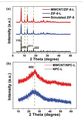
**Fig. 2** XRD patterns of (a) as-synthesized MWCNT/ZIF-8-L, ZIF-8-L, (b) MWCNT/NPC-L, NPC-L.
