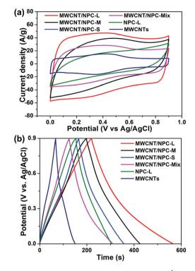
**Fig. 7** (a) CV curves at a potential scan rate of 200 mV s<sup>-1</sup>. (b) Charge– discharge curves at a current density of 1 A g<sup>-1</sup> for MWCNT/NPC-S/M/L, MWCNT/NPC-Mix, NPC-L and MWCNTs.
