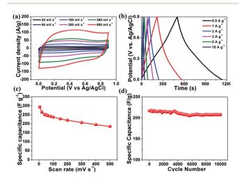
**Fig. 8** (a) CV curves at different scan rates. (b) Charge–discharge curves at current densities ranging from 0.5 to 10 A g<sup>-1</sup>. (c) Specific capacitance curves at the different scan rates from 20 to 500 mV s<sup>-1</sup>. (d) Variation of the specific capacitance within 10 000 cycles at the scan rate of 100 mV s<sup>-1</sup>.
