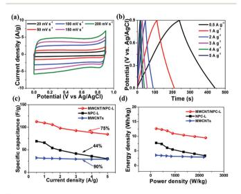
Fig. 10 Electrochemical performances evaluated by symmetrical twoelectrode supercapacitors in 1 M  $H_2SO_4$  solution. (a) CV curves of MWCNT/NPC-L-based SSC at different scan rates. (b) Charge-discharge curves of MWCNT/NPC-L-based SSC at various current densities. (c) Specific capacitance under different current densities from 0.5 to 5 A g<sup>-1</sup>. (d) Ragone plot for the SSCs based on MWCNT/NPC-L, NPC-L and MWCNTs under various current densities.
