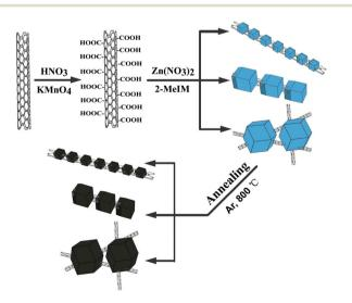
Fig. 1 Synthetic scheme for the fabrication of MWCNT/NPC-S/M/L.
