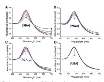
Fig. 4 Assessment of specificity of thermally gated nanoparticles to a panel of lectins. Lectin concentration is  $1-10 \mu g mL^{-1}$ . (A-D) Show UV-Visible traces (normalised to Abs<sub>450</sub>) following 30 minutes incubation at 40 °C with indicated lectin. Arrow indicates increase concentration.
