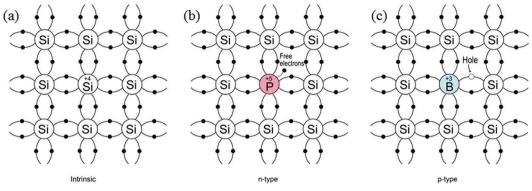
Schematic bond representation for (a) intrinsic silicon; (b) n-type silicon doped with phosphorus and (c) p-type silicon doped with boron.
