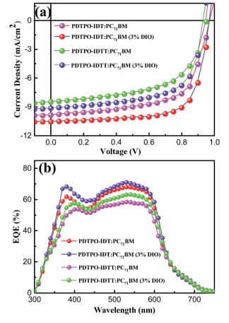
Fig. 4 (a) J-V characteristics curves of PDTPO-IDT:  $PC_{71}BM$  (1: 2, w/w) and PDTPO-IDTT:  $PC_{71}BM$  (1: 2, w/w) based PSCs without or with 3% DIO (v/v) under AM 1.5 G at 100 mW cm<sup>-2</sup>. (b) Corresponding EQE spectra of PDTPO-IDT:  $PC_{71}BM$  and PDTPO-IDTT:  $PC_{71}BM$  based PSCs without or with 3% DIO (v/v).
