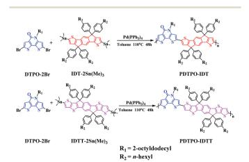
Scheme 1 Synthesis and chemical structures of PDTPO-IDT and PDTPO-IDTT.
