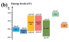
Fig. 2 (a) The electrochemical cyclic voltammetry measurements of PDTPO-IDT and PDTPO-IDTT thin film coated on the platinum electrode in acetonitrile solution containing  $0.1\,\mathrm{M\,n\textsc{-}Bu_4NPF_6}$  at a scan rate of 100 mV s<sup>-1</sup>. (b) Schematic energy level diagram of all components used in conventional devices.
