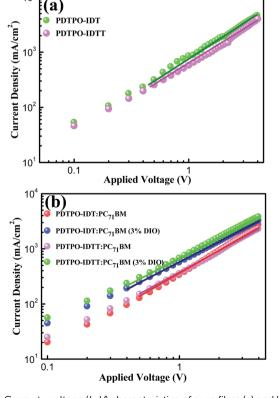
Fig. 5 Current–voltage (I-V) characteristics of pure films (a) and blend films (b) (with or without 3% DIO) PDTPO-IDT: PC<sub>71</sub>BM (1:2, w/w) and PDTPO-IDTT: PC<sub>71</sub>BM (1:2, w/w) in space-charge-limited current (SCLC) devices.
