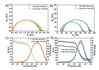
Fig. 7 EIS spectra of aqueous DSSCs assembled with KI 1.50 M + I<sub>2</sub> 50 mM (A and C) and NaI 1.50 M + I<sub>2</sub> 50 mM (B and D). Data points were fitted (lines) according to eqn (3) with the constraints  $R_{\rm Pt}=2~\Omega$  and  $C_{\rm Pt}=2~\times~10^{-5}~{\rm F}$ .
