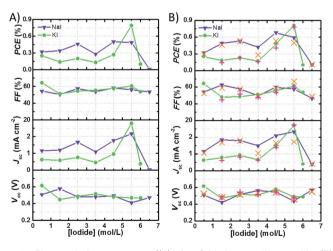
Fig. 4 Photovoltaic parameters ((A) after 24 h from cell assembly, (B) best value recorded in the cell lifetime) of aqueous DSSCs bearing different I $^-$  concentrations (I $_2$  50 mM). Orange crosses (×) or red plus signs (+) correspond to the average values at the given NaI or KI concentrations, respectively. Lines simply connect data points and have no physical meaning. Cells were tested under 1 sun irradiation and the reported data were recorded at the  $3^{\rm rd}\,J{-}V$  measurement.
