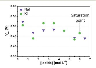
Fig. 3 Average  $V_{\rm oc}$  values recorded one day after cell assembly. I<sub>2</sub> was kept constant at 50 mM for all the cells. Data are referred to the 3<sup>rd</sup> measurement under 1 sun irradiation. Data referred to the electrolytes saturated with KI were arbitrarily placed at 6 M.
