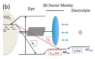
Fig. 1 Utilization of intramolecular hole transfer to enhance dye cation regeneration. (a) Reduced recombination and slower regeneration kinetics; (b) faster dye regeneration kinetics at a smaller driving force using a tridimensional donor moiety.
