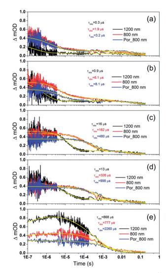
Fig. 7 Transient absorption decay and fitted curves of  $TiO_2$ –Por–(Cb–TPA) probed at 1200 nm (black) and 800 nm (red) and  $TiO_2$ –Por probed at 800 nm (blue) with five  $I^-/I_3^-$  electrolytes after pulsed 532 nm laser irradiation. (a)  $I_-1$ , (b)  $I_-0.1$ , (c)  $I_-0.01$ , (d)  $I_-0.001$  and (e)  $I_-0.01$ , (f)  $I_-0.001$  and (e)  $I_-0.001$  nm, 45–50  $I_-0.001$  per pulse; repetition rate 1 Hz).
