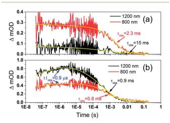
Fig. 6 Transient absorption decays and fitted functions of (a)  $TiO_2$ –Por and (b)  $TiO_2$ –Por–(Cb-TPA) with the inert electrolyte I\_0 (532 nm,  $45-50 \mu J$  cm<sup>-2</sup> per pulse; repetition rate 1 Hz).
