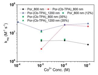
Fig. 9 Regeneration rate constant of Por and Por–(Cb-TPA) versus the concentration of  ${\rm Co}^{2+}$ . Por with 12% dye-loading probed at 800 nm and Por–(Cb-TPA) with 35% dye-loading probed at 800 nm and 1200 nm are also shown.
