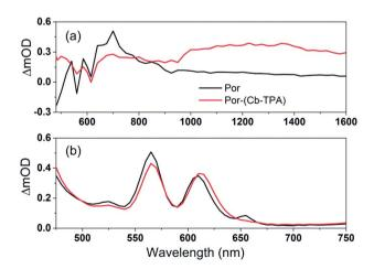
Fig. 5 (a) Transient absorption spectra of  $TiO_2$ –Por and  $TiO_2$ –Por–(Cb-TPA) in the presence of the inert electrolyte I\_0 at 10  $\mu$ s time delay following laser excitation (532 nm, 24–26  $\mu$ J cm<sup>-2</sup> per pulse) and (b) absorbance of  $TiO_2$ –Por and  $TiO_2$ –Por–(Cb-TPA).
