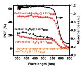
Fig. 3 IPCE of raw- $Ta_3N_5$  (orange), necked- $Ta_3N_5$  (black) and CoPi/necked- $Ta_3N_5$  (red) electrodes. The absorption spectrum (black solid curve) for raw  $Ta_3N_5$  is presented for comparison.
