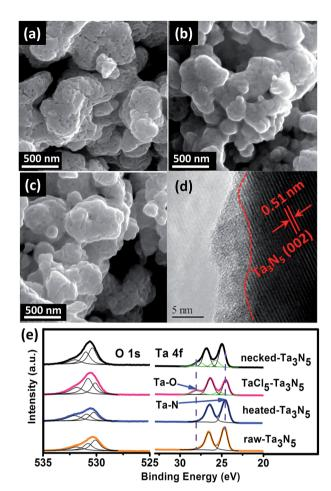
Fig. 1 SEM images of (a) raw- $Ta_3N_5$  electrode, (b)  $TaCl_5-Ta_3N_5$  electrode, and (c) necked- $Ta_3N_5$  electrode. (d) HRTEM image of necked- $Ta_3N_5$  electrode. (e) XPS spectra of O 1s and Ta 4f for raw- $Ta_3N_5$  (orange), heated- $Ta_3N_5$  (blue),  $TaCl_5-Ta_3N_5$  (pink) and necked- $Ta_3N_5$  (black) electrodes.
