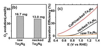
Fig. 4 (a) Schematic comparison of  $O_2$  evolution processes via photocatalysis (AgNO $_3$  as electron scavenger) and photoelectrocatalysis. (b) Photocatalytic activity of the  $Ta_3N_5$  powder peeled from raw- $Ta_3N_5$  and necked- $Ta_3N_5$  electrodes. The mass of the photocatalyst is listed above the column, respectively. (c) Charge separation efficiency of raw- $Ta_3N_5$  (orange), necked- $Ta_3N_5$  (black) and CoPi/necked- $Ta_3N_5$  electrodes (red).
