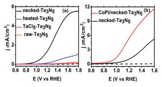
Fig. 2 Current–potential (j-E) curves of (a) raw-Ta<sub>3</sub>N<sub>5</sub> (orange), TaCl<sub>5</sub>–Ta<sub>3</sub>N<sub>5</sub> (pink), heated-Ta<sub>3</sub>N<sub>5</sub> (blue), necked-Ta<sub>3</sub>N<sub>5</sub> (black) and (b) CoPi/necked-Ta<sub>3</sub>N<sub>5</sub> (red) electrode. Electrolyte: 1 M NaOH aqueous solution. Illumination: 100 mW cm<sup>-2</sup>. AM 1.5 G.
