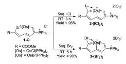
Scheme 2 Reactions of osmapentalyne 1-Cl with ICl and  $Br_2$ .
