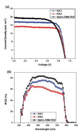
Fig. 4 (a) J-V characteristics of the solar cells with HA1, HA2 and spiro-OMeTAD as the HTM. (b) The IPCE spectra of characteristics of the perovskite solar cells with HA1, HA2 and spiro-OMeTAD as the HTM.
