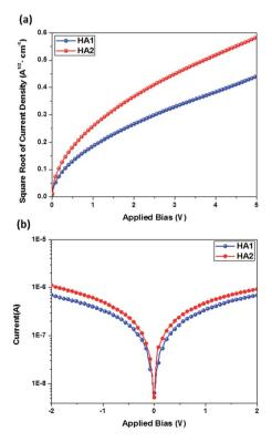
Fig. 3 (a) J-V plots of the hole-only devices based on HA1 and HA2. (b) Conductivity characteristics of devices based on HA1 and HA2.
