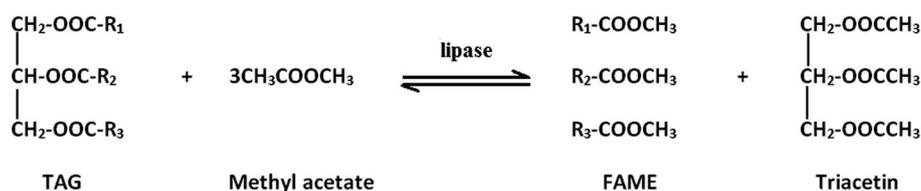
Fig. 3 Interesterification reaction of TAG with methyl acetate producing FAME and triacetin as by-product.<sup>81</sup>
