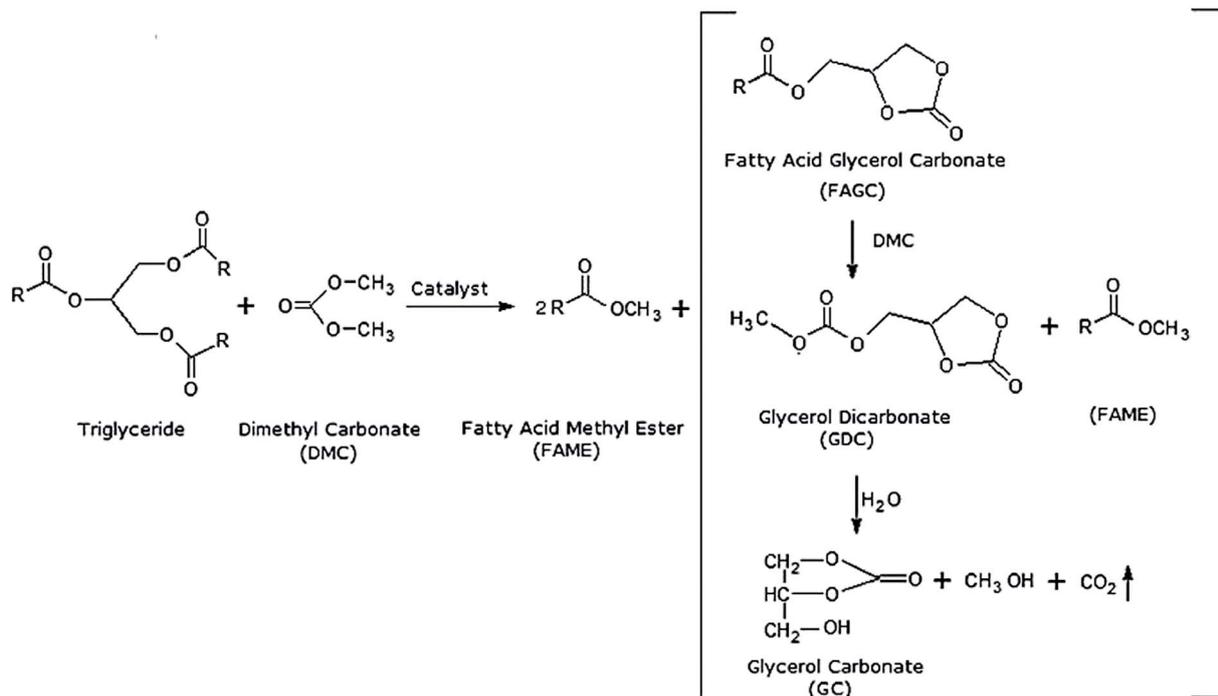
Fig. 4 Interesterification of triglyceride with dimethyl carbonate (DMC) producing FAME and Fatty Acid Glycerol Carbonate (FAGC).<sup>89</sup> FAGC will be further broken down into glycerol dicarbonate (GDC) and glycerol carbonate (GC).
