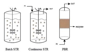
Fig. 5 Reactor design: batch STR (stirred tank reactor), continuous STR, and PBR (packed bed reactor).<sup>53</sup>
