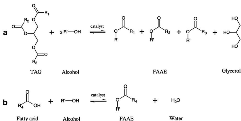
Fig. 2 Reactions for synthesis of fatty acid alkyl ester (FAAE).<sup>11</sup> (a) Transesterification of TAG (triacylglyceride) with alcohol producing FAAE and glycerol as by-product. (b) esterification of fatty acid with alcohol producing FAAE and water as by-product. R<sub>1-4</sub> are acyl residues, R' is alcohol moiety.
