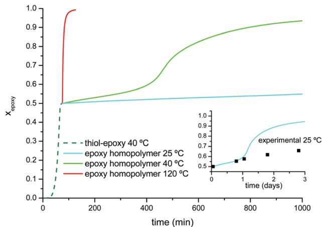
**Fig. 5** Simulation of curing schedules of formulation DG174S3-0.5 using the isoconversional kinetics data. The inset shows the extended simulation of the second stage of the curing at 25 °C with a timescale of days; the square symbols are experimental points corresponding to samples kept in a silicone oil bath at 25 ± 0.5 °C.
