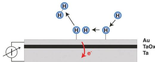
**Fig. 1** Principle of the application of thin metal film devices for the study of coupling to electronic degrees of freedom in surface chemistry. The chemistry proceeding on the front side goes along with the excitation of electron–hole-pairs, the electrons of which may in this case pass the barrier imposed by the oxide layer, provided they have sufficient energy. The resulting electron flux can externally be detected as a macroscopic current.
