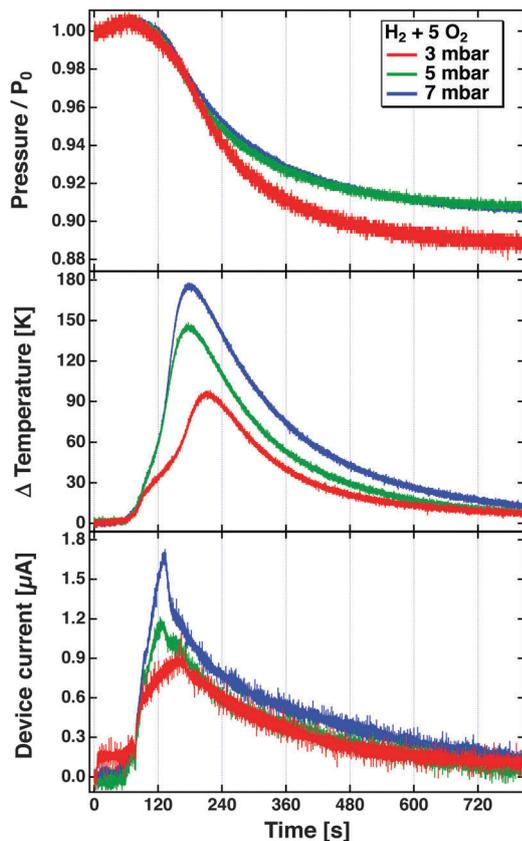
Fig. 8 Pressure, temperature increase and device current observed during the reaction of  $\text{H}_2$  with  $\text{O}_2$  in a bulb experiment using a Pt/Si device. The bulb (55l) was filled with  $\text{H}_2$  and  $\text{O}_2$  in the ratio of 1:5 to total pressures of 3, 5 and 7 mbar. The reaction was initiated at about  $t = 80$  s by irradiating the Pt surface with a light bulb which causes the temperature to rise from room temperature to the ignition temperature.<sup>81</sup>
