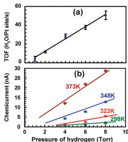
Fig. 6 (a) Turnover frequency for different pressures of H<sub>2</sub> in  $10^5 \text{ Pa}$  of O<sub>2</sub> at 353 K. (b) A plot of the chemicurrent as a function of different H<sub>2</sub> pressures in  $10^5 \text{ Pa}$  of O<sub>2</sub>. Reprinted with permission from ref. 74. Copyright (2009) American Chemical Society.
