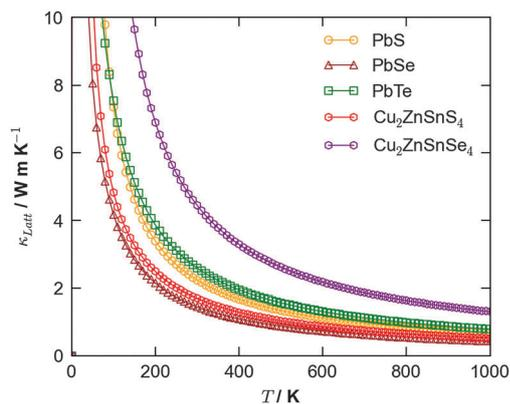
Fig. 3 Calculated lattice thermal conductivity using anharmonic lattice dynamics as a function of temperature for the binary lead chalcogenides, PbS, PbSe and PbTe,<sup>38</sup> and the quaternary semiconductors Cu<sub>2</sub>ZnSnS<sub>4</sub> and Cu<sub>2</sub>ZnSnSe<sub>4</sub>.<sup>40</sup>
