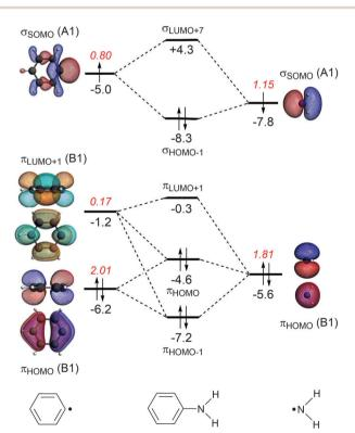
Fig. 1 MO diagrams for the C-N bond formation from Ph\* and \*NH2 into aniline with the electron-pair formation in the  $\boldsymbol{\sigma}$  system (only A1 orbitals) at the top and the donor-acceptor interactions in the  $\pi$  system (only B1 orbitals) at the bottom. The energies (eV) of the molecular or fragment orbitals are given in black and the gross electron population of the fragment orbitals in red.
