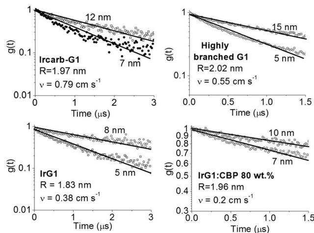
Fig. 3 Ratio of the phosphorescence intensity  $g(t)$  measured for thin films of given thicknesses on fused silica substrates to that of the limiting case of a thick film. Solid lines are fits to an exponential decay and the values of the surface quenching velocities  $\nu$  obtained using eqn (3) are given for each material as insets.  $R$  is the average intermolecular spacing between the iridium(III) complex cores.
