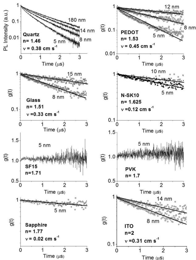
Fig. 6 Ratio of the phosphorescence intensity  $g(t)$  measured for neat thin films of IrG1 of given thicknesses to that in the thick film on different substrates,  $n$  is the refractive index of the substrate at the PL peak. Solid lines are fits to an exponential decay and surface quenching velocities  $v$  obtained using eqn (3) are given.
