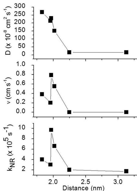
Fig. 4 Triplet exciton diffusion coefficient  $D$ , surface quenching velocity  $v$  of the thin films, and the non-radiative decay rate  $k_{\text{NR}}$  in the bulk films as a function of the intermolecular distance between complexes  $R$ .
