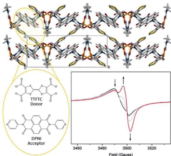
**Fig. 3** The charge transfer MOF  $[(\text{Zn}(\text{DMF})_2)(\text{TTFTC})(\text{DPNI})]$  which exhibits through-space CT interactions. Reduction of the MOF switches the CT off. This is consistent with solid state EPR spectroelectrochemistry which revealed evidence for a concomitant decrease in the TTFTC radical cation, and an increase in the DPNI radical anion signal, thus reducing the donor-acceptor interaction. Reproduced from ref. 62 with permission from the Royal Society of Chemistry.
