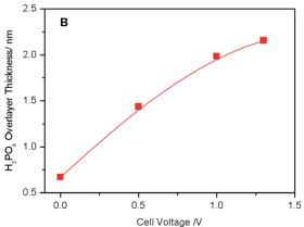
Fig. 3 (A) Pt/O and Pt/P atomic ratios normalized to the corresponding values at the OCV (black left-hand-side axis), and LBE ( $O_{LBE}$ ) to HBE ( $O_{HBE}$ ) oxygen intensity (red right-hand-side axis) obtained via deconvolution of spectra presented in Fig. 2B as a function of the cell voltage. (B) Apparent thickness of the PA film calculated as a function of the applied cell voltage.
