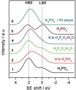
Fig. 4 Simulated O 1s XP spectra for various molecular/ionic configurations using convolution of Gaussian shape peaks with relative BE shifts calculated by means of the DFT. For more details see the ESI.†
