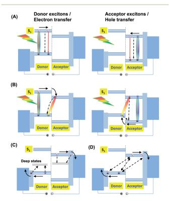
Fig. 7 Schematic depictions of the generation of donor excitons and acceptor excitons, electron and hole transfer, and loss mechanisms *via* exciton decay (A), recombination of bound electron—hole pairs (B), and recombination of mobile electrons and holes as trapped by deep states (C) or in a bimolecular mechanism (D).
