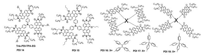
Fig. 11 Chemical structures of the PDI trimer and tetramer acceptors.
