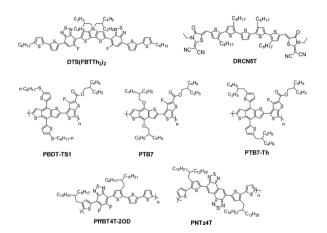
Fig. 2 The molecular structures of typical small-molecule and polymer donors from which a PCE of 10-11% or 11-12% has been realized for single-junction or tandem solar cells. The molecules are reported as follows: PTB7 ( $E_q^{opt} = 1.63 \text{ eV}$ ), <sup>22</sup> PTB7-Th (1.58 eV), <sup>23</sup> DTS(FBTTh<sub>2</sub>)<sub>2</sub> (1.55 eV),<sup>24</sup> DRCN5T (1.60 eV),<sup>25</sup> PBDT-TS1 (1.51 eV),<sup>26</sup> PffBT4T-2OD (1.55 eV).5 and PNTz4T (1.54 eV).34
