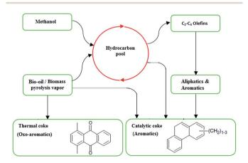
Fig. 10 Kinetic scheme suggested for the bio-oil/biomass and methanol mixture conversion into hydrocarbons and coke on HZSM-5 catalysts. Adapted from Valle et al. 115
