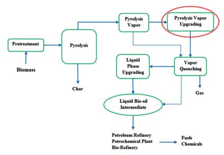
Fig. 2 Schematic of pyrolyis process and upgrading – highlighting pyrolysis vapor upgrading
