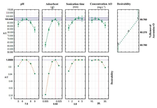
Fig. 6 Profiles for predicated values and desirability function for removal percentage of AO. Dashed line indicated current values after optimization.
