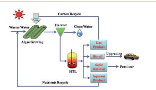
Fig. 11 Concept of Environment-Enhancing-Energy (E<sup>2</sup>-Energy) technology. 42 Copyright 2011 Royal Society of Chemistry.
