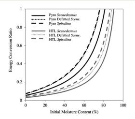
Fig. 18 ECR for HTL and pyrolysis of algal biomass at varying initial moisture contents.<sup>86</sup> Copyright 2012 Elsevier.
