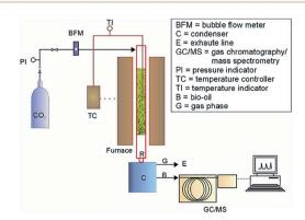
Fig. 5 Schematic reactor system for microalgae pyrolysis.<sup>56</sup> Copyright 2012 Elsevier.
