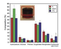
Fig. 7 Bio-oil composition of pyrolysis employed at three atmospheres: N<sub>2</sub>, steam, and CO<sub>2</sub> (ref. 111). Copyright 2012 Elsevier. Process conditions: 773 K,  $N_2$  flow = 250 mL min<sup>-1</sup>, algae mass = 7 g, dp < 90 mm.
