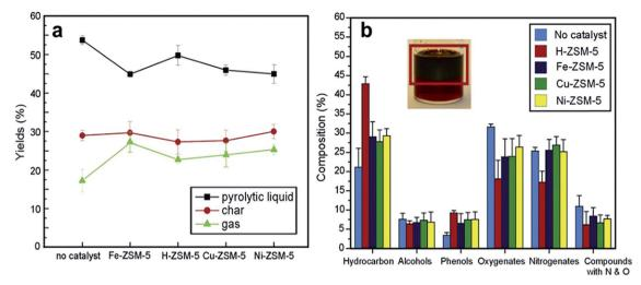
Fig. 8 Experimental results of catalytic pyrolysis reactions conducted using different zeolites. <sup>111</sup> Copyright 2012 Elsevier. (a) Effect of catalyst on product yield in catalytic pyrolysis reactions. (b) Bio-oils product distribution. Process conditions: 773 K,  $N_2$  flow = 250 mL min<sup>-1</sup>, algae mass = 7 g, WHSV = 13.5 h<sup>-1</sup>, GHSV = 20 000 h<sup>-1</sup>, residence time  $\sim$ 1.5 s.
