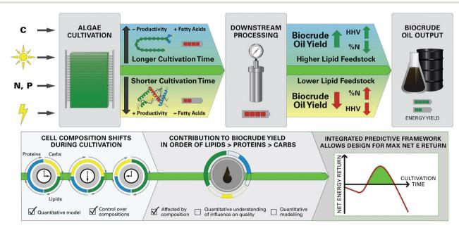
Fig. 1 The integrated modeling framework allows for prediction and optimization of system-scale parameters for the microalgae-HTL biofuel system. The top half of the figure represents the integrated processing scheme for microalgae HTL, with the black arrows representing decisions on cultivation times that lead to downstream implications. The bottom half represents the current research progress towards formulating an integrated
