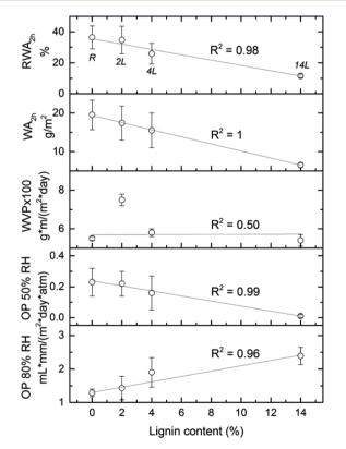
Fig. 10 Relative water absorption of the nanopapers after 2 h of immersion in water (RWA2h), water absorption (WA2h) and barrier properties (WVP and OP) of the nanopapers evaluated as a function of the lignin content.
