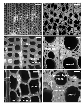
Fig. 2 Low-vacuum scanning electron microscopy of microtome cross-sections of spruce (A, C, E) and beech (B, D, F) CaCO $_3$  composites prepared at [DMC] = [CaCl $_2$ ] = 1.5 mol L $^{-1}$  prior to drying. SEM images in the backscattered electron mode give evidence of relatively void lumina and depositions of electron-dense material along middle lamellae and rays, within beech fibres and parenchyma cells. Scale-bars correspond to 500  $\mu$ m (A, B), 100  $\mu$ m (C, D) and 20  $\mu$ m (E, F).
