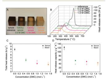
Fig. 4 (A) Photo of native spruce and spruce/CaCO<sub>3</sub> composites after heat treatment in a muffle furnace (20 min, 250 °C). (B) Typical temperaturedependent heat release rate curves from pyrolysis combustion flow calorimetry (PCFC) of beech samples after base-line correction. The key parameters total heat release (C) and heat release capacity (D) of spruce and beech are plotted as a function of the precursor concentration [DMC] = [CaCl<sub>2</sub>].
