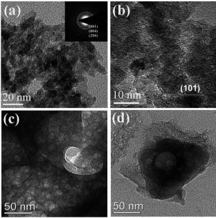
Fig. 6 (a) TEM image and (b) HRTEM image of  $TiO_2$  with wormhole mesopores. <sup>98</sup> (c and d) TEM images of porous  $Li_3V_2(PO_4)_3/C$ . <sup>61</sup> (c and d) Adopted from ref. 61, Copyright 2012, with permission from Elsevier.
