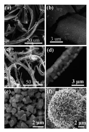
Fig. 5 SEM images of the ZnO post-annealing at 600 °C (a and b),  $^{85}$  SrAl<sub>x</sub>O<sub>y</sub> post-annealing at 1300 °C (c and d),  $^{86}$  triangular ZnO (e),  $^{87}$  and CuO nanoflowers (f).  $^{88}$  (e) Adopted from ref. 87, Copyright 2009, with permission from American Chemical Society. (f) Adopted from ref. 88, Copyright 2013, with permission from Elsevier.
