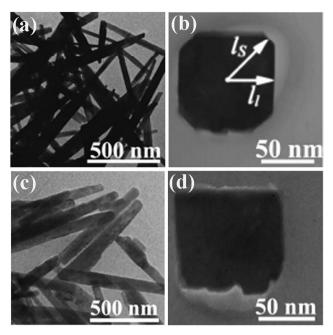
Fig. 4 TEM images of (a and b) Al<sub>4</sub>B<sub>2</sub>O<sub>9</sub> nanowires synthesized at 900  $^{\circ}$ C for 2 h and (c and d) Al<sub>18</sub>B<sub>4</sub>O<sub>33</sub> nanowires synthesized at 1050  $^{\circ}$ C for 2 h.84 Adopted from ref. 84, Copyright 2007, with permission from American Chemical Society.
