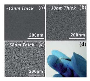
Fig. 11 (a–c) SEM images of  $In_2O_3$  films on n++ Si with controlled thickness. (d) Optical image of a flexible combustion-processed  $In_2O_3$  device.<sup>51</sup> Adopted from ref. 51, Copyright 2011, with permission from Macmillan Publishers Ltd.
