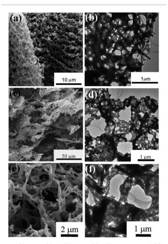
Fig. 9 SEM image (a) and TEM image (b) of 3D macroporous NiO/Ni. SEM image (c) and TEM mage (d) of 2D macroporous NiO/Ni.<sup>115</sup> SEM image (e) and TEM image (f) of 3D porous ZnO. 116 (a-d) Adopted from ref. 115, Copyright 2013, with permission from Elsevier.
