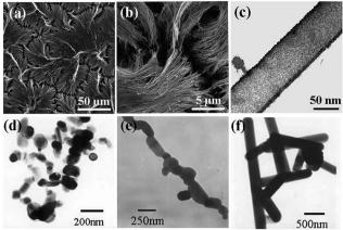
Fig. 3 SEM (a, b) and TEM (c) images of hydroxyapatite nanotubes.<sup>79</sup> TEM images of Caln<sub>2</sub>O<sub>4</sub>: (d) as-combusted, (e) post-annealed at 1373 K for 2 h and (f) post-annealed at 1373 K for 12 h.80 (a-c) adopted from ref. 79, Copyright 2008, with permission from Elsevier. (d-f) adopted from ref. 80, Copyright 2009, with permission from Springer.
