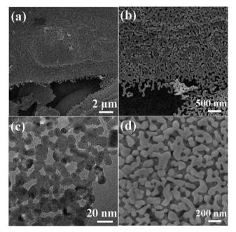
Fig. 8 (a and b) SEM images of porous ZnO network. <sup>110</sup> (c) TEM image of mesoporous  $Co_3O_4$  calcined at 355 °C. <sup>111</sup> (d) SEM image of macroporous  $Co_3O_4$  calcined at 550 °C. <sup>111</sup> (a and b) Adopted from ref. 110, Copyright 2012, with permission from AIP Publishing.
