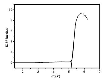
Fig. 1 Kubelka–Munk-transformed diffuse reflectance spectra of ZIF-8.
