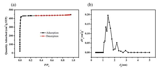
Fig. 2 (a) N<sub>2</sub> adsorption-desorption isotherms of ZIF-8 at 77 K. (b) Micro-pore size distribution of ZIF-8.
