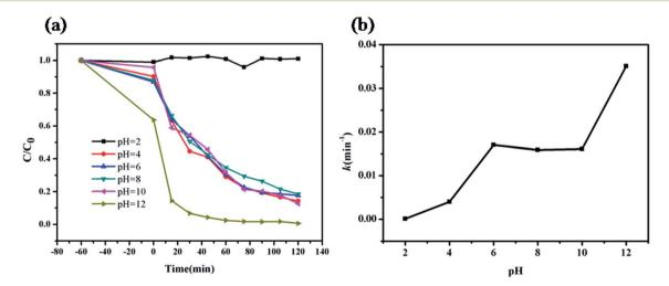
Fig. 5 (a) Effect of initial pH on the degradation of MB. Experimental conditions: ZIF-8, 0.5 g  $L^{-1}$ ; MB, 10 mg  $L^{-1}$  and UV irradiation. (b) The corresponding pseudo-first-order rate constants for system with pH = 2.0-12.0.
