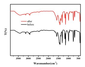
Fig. 8 FTIR spectra of ZIF-8 before and after photocatalytic reaction.
