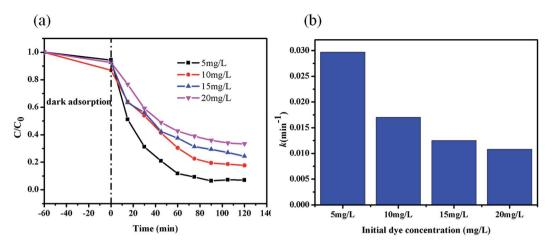
Fig. 4 (a) Effect of initial dye concentration on the degradation of MB. (b) Comparison of the apparent rate constants of the degradation of MB with different initial concentrations. Experimental conditions: ZIF-8, 0.5 g  $L^{-1}$  and UV irradiation.
