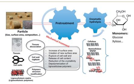
Fig. 3 Different steps of biomass conversion and parameters influencing lignocellulosic particle reactivity.
