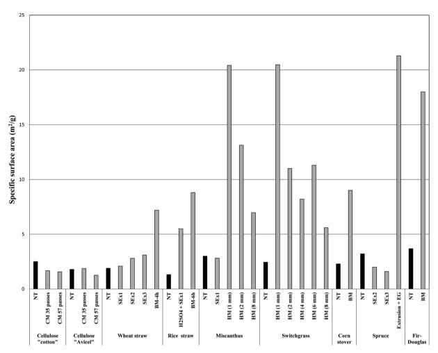
Fig. 4 Effect of mechanical size reduction on specific surface area (SSA) of selected lignocellulosic biomass compared to others pretreatments. NT: not treated; CM: compression milling; BM: ball milling; HM: hammer milling; SEx: steam explosion; EG: ethylene glycol.
