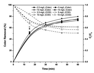
Fig. 1 Effect of ferric ion concentration on color and COD removal in the EF process at solution pH 3 and applied voltage of 3.5 V.
