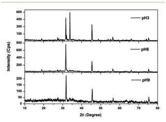
XRD spectra of sludge produced at various solution pHs.
