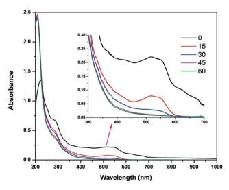
Fig. 6 Changes in UV-visible spectra of textile wastewater at applied voltage of 7 V, pH 3 and ferric ion concentration of 10 mg  $\rm L^{-1}$ .
