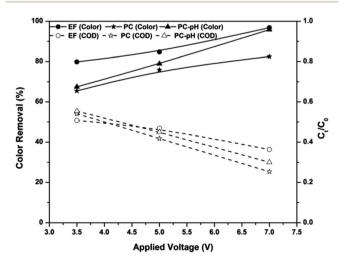
Fig. 2 Effect of applied voltage on COD and color removal efficiencies of the EF, PC and PC-pH processes at pH 3, ferric ion dosage of  $10 \text{ mg L}^{-1}$ , electrode area of  $25 \text{ cm}^2$ .
