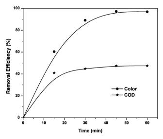
Fig. 10 Color and COD removal kinetics of the EF process in the presence of sludge as heterogeneous catalyst at pH  $^{3}$  and applied voltage of 7 V.
