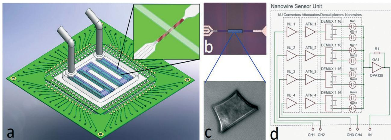
**Fig. 6** (a) CAD design of the 64 NW sensor with microfluidics channel. The inset shows the microchannel crossing over the nanowire array. (b) A microscope photograph of fabricated 4 NW sensors. (c) A TEM image of a NW cross section. Inset scale bar is 20 nm long. (d) A circuit diagram of voltage-based interrogation with an option to measure 64 NW sensors.
