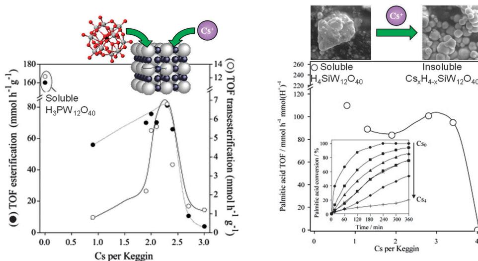
Fig. 10 Impact of Cs ion-exchange into (left) both  $\text{Cs}_x\text{H}_{(3-x)}\text{PW}_{12}\text{O}_{40}$  for palmitic acid esterification and tributyrin transesterification with methanol; and (right) and  $\text{Cs}_y\text{H}_{(4-y)}\text{SiW}_{12}\text{O}_{40}$  for palmitic acid esterification, benchmarked against parent fully protonated, soluble clusters. Adapted from ref. 138 and 177. Copyright (2007 and 2009), with permission from Elsevier.
