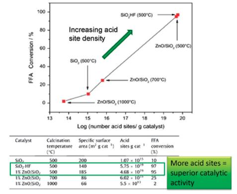
Fig. 8 Relationship between acid site density and catalytic performance in FFA esterification. Adapted from ref. 171. Copyright (2014), with permission from Elsevier.
