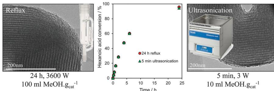
Fig. 9 Surfactant template extraction *via* energy/atom efficient ultrasonication delivers a one-pot  $\text{PrSO}_3\text{H-SBA-15}$  solid acid catalyst with identical structure and reactivity to that obtained by conventional, inefficient reflux. Adapted from ref. 172 with permission from The Royal Society of Chemistry.
