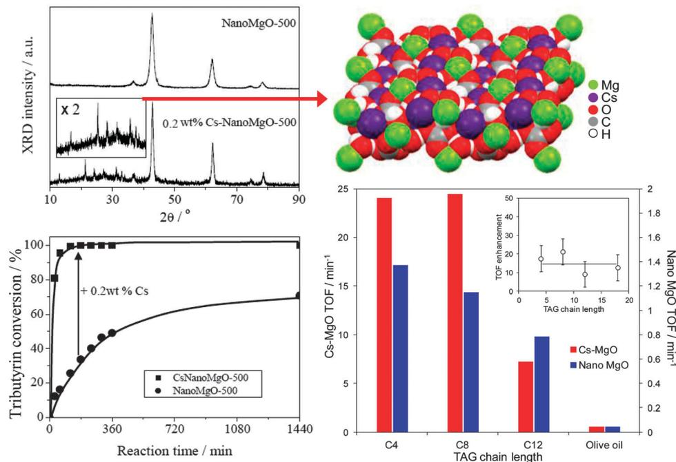
Fig. 2 Formation of crystalline  $\text{Cs}_2\text{Mg}(\text{CO}_3)_2(\text{H}_2\text{O})_4$  phase within co-precipitated Cs-doped MgO and resulting synergy in the transesterification of short and long chain TAGs with methanol compared with undoped nanocrystalline MgO. Adapted from ref. 85 with kind permission from Springer Science and Business Media and ref. 92 with permission from John Wiley and Sons.
