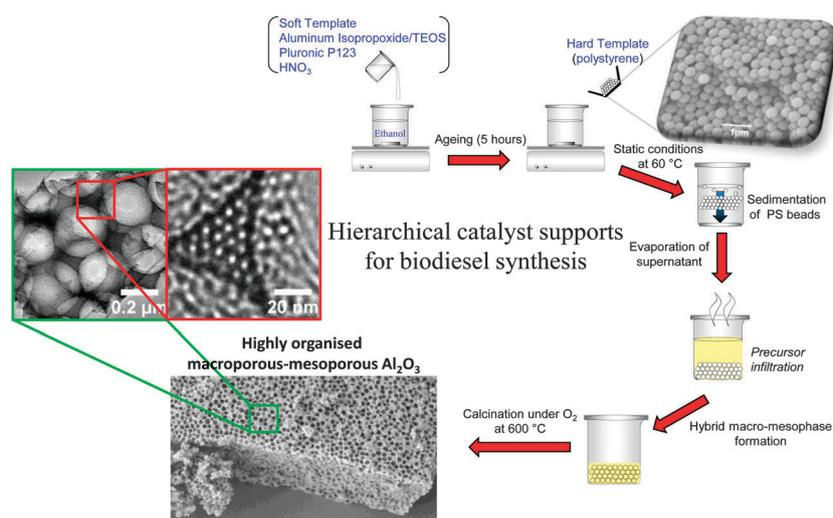
Scheme 4 Liquid crystal and polystyrene nanosphere dual surfactant/physical templating route to hierarchical macroporous–mesoporous silicas.
