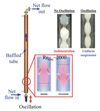
Fig. 18 Schematic of reactor flow and mixing characteristics within an OBR, and associated optical images of a PrSO<sub>7</sub>H-SBA-15 solid acid powder without oscillation (undergoing sedimentation) or with a 4.5 Hz oscillation (entrained within baffles). Adapted from ref. 42 with permission from The Royal Society of Chemistry
