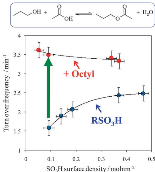
Fig. 16 (left) Molecular dynamics simulations of MCM- $\text{SO}_3\text{H}$  and MCM-Oc- $\text{SO}_3\text{H}$  pore models highlighting the interaction between surface sulfonic acid and hydroxyl groups in the absence of co-grafted octyl chains; (right) influence of  $\text{PrSO}_3\text{H}$  surface density and co-grafted octyl groups on catalytic performance in acetic acid esterification with butanol. Adapted from ref. 213 with permission from The Royal Society of Chemistry.
