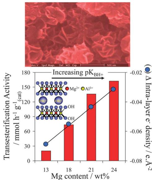
Fig. 5 Impact of Mg:Al hydrotalcite surface basicity on their activity towards tributyrin transesterification. Adapted from ref. 117. Copyright (2005), with permission from Elsevier.
