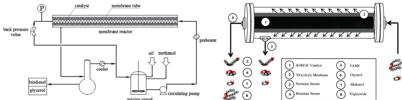
**Fig. 19** Schematic of recirculating packed membrane reactors for continuous biodiesel production *via* (a) solid acid and (b) base catalysts. Reprinted from ref. 252 and 254. Copyright (2011 and 2014), with permission from Elsevier.
