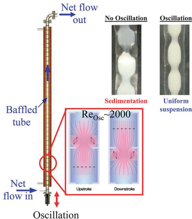
**Fig. 18** Schematic of reactor flow and mixing characteristics within an OBR, and associated optical images of a  $\text{PrSO}_3\text{H-SBA-15}$  solid acid powder without oscillation (undergoing sedimentation) or with a 4.5 Hz oscillation (entrained within baffles). Adapted from ref. 42 with permission from The Royal Society of Chemistry.
