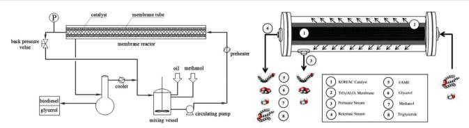
Fig. 19 Schematic of recirculating packed membrane reactors for continuous biodiesel production via (a) solid acid and (b) base catalysts. Reprinted from ref. 252 and 254. Copyright (2011 and 2014), with permission from Elsevier.
