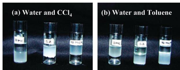
Fig. 17 Preferential dispersion of DMC in the nonpolar, organic phase, and SZ and Al-MCM-41 in the polar aqueous phase of (a) water- $\text{CCl}_4$  and (b) water-toluene solvent mixtures. Reprinted with permission from ref. 202. Copyright 2010 American Chemical Society.
