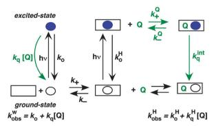
Scheme 5 Representation of the mechanism where the excited state (blue solid circle) is too short lived to interchange between the solvent and the host (square). Quenching reactions are shown is green.
