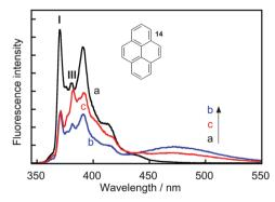
Fig. 7 Fluorescence spectra for pyrene (14,  $0.5 \mu M$ ) in water (a, black) and in the presence of 5 mM (b, blue) and 20 mM (c, red)  $\gamma$ -cyclodextrin. (Adapted with permission from A. S. M. Dyck, U. Kisiel and C. Bohne, J. Phys. Chem. B, 2003, 107, 11652-11659. Copyright 2003 American Chemical Society.)
