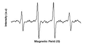
Fig. 4 Spectrum of DMPO-OH derived from ZnO NP coating in the presence of the spin trap, DMPO.
