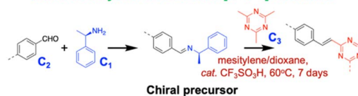
Scheme 1 (a) Previously reported chirality-induced transamination via a reversible aldimine condensation reaction. (b) Currently used chirality-induced imine-to-vinylene conversion via an irreversible aldol condensation reaction. Reaction conditions: 60 °C, 7 days, CF_3SO_3H (catalyst), mesitylene/dioxane (1/1, v/v).
