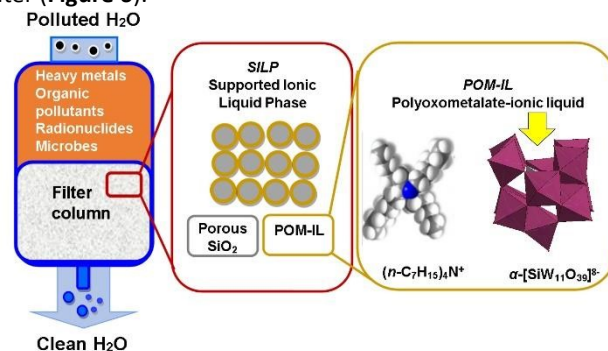
Figure 6. Water purification using POM-SILPs: the POM-SILP column filter removes toxic heavy metals (e.g. Ni(II) , Pb(II) , UO_2(II) ), microbes ( E. coli ), and aromatic organic pollutants (e.g. trityl dyes) due to the presence of lacunary polyoxometalate anions with specific metal-binding sites (yellow arrow) and antimicrobial tetra-alkyl ammonium cations. Reproduced from Ref. 63 with permission from Wiley-VCH, Copyright 2017.
