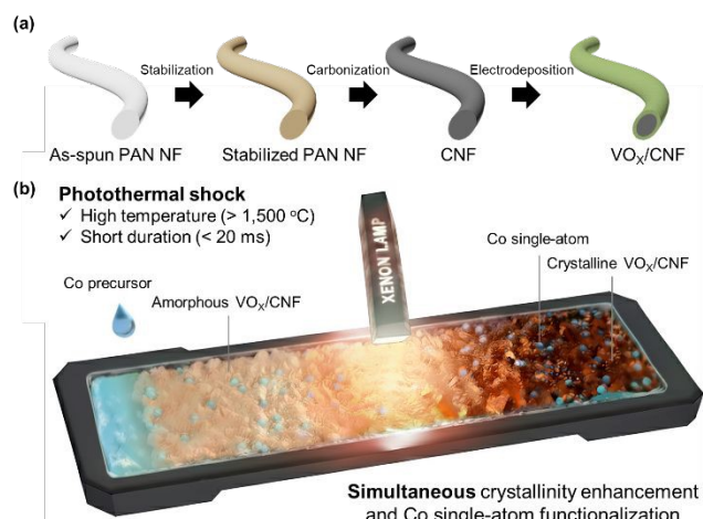
Fig. 1 (a) Schematic illustration of fabrication of amorphous \text{VO}_x on CNF. (b) Schematic illustration of the synthesis of \text{Co}/\text{VO}_x/\text{CNF} via ultrafast photothermal shock process, highlighting the simultaneous crystallinity enhancement and Co single-atom anchoring.
