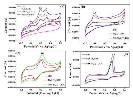
Fig. 6 Cyclic voltammograms of LIG, Ti<sub>3</sub>C<sub>2</sub>T<sub>x</sub>/LIG and NiO-Ti<sub>3</sub>C<sub>2</sub>T<sub>x</sub>/LIG electrodes in 0.1 M PBS (pH 7.4) containing (a) a mixture of 2 mM AA, 1 mM DA and 1 mM UA, (b) 2 mM AA, (c) 1 mM DA and (d) 1 mM UA at a scan rate of 10 mV s<sup>-1</sup> compared to the response with only buffer solution.
