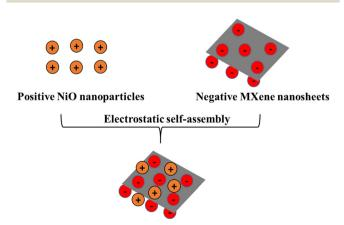
Fig. 1 Schematic illustration of the fabrication of the NiO-Ti<sub>3</sub>C<sub>2</sub>T<sub>x</sub> MXene composite.
