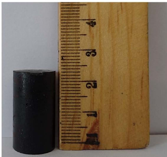
Fig. 3 Specimen used for the compressive strength test.
