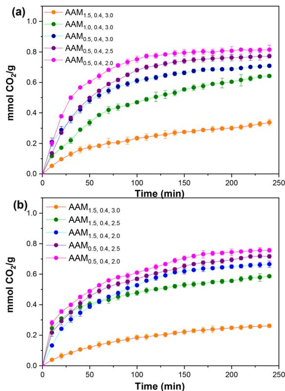
Fig. 10 CO<sub>2</sub> uptake profiles of AAMs at (a) 7 and (b) 28 days (error bars are standard errors).
