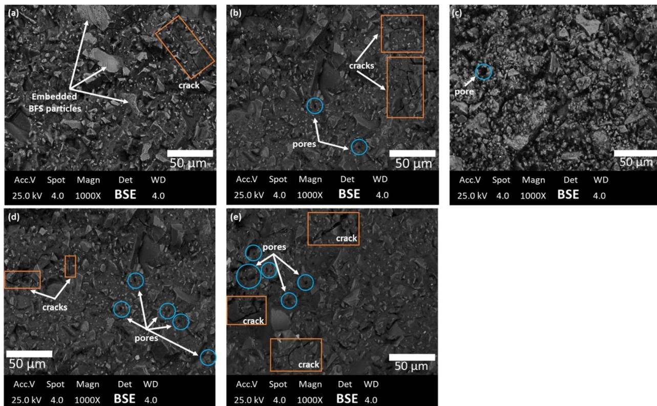
Fig. 7 Backscattered electron image of (a)  $AAM_{1.5, 0.4, 3.0}$ , (b)  $AAM_{1.0, 0.4, 3.0}$ , (c)  $AAM_{0.5, 0.4, 3.0}$ , (d)  $AAM_{0.5, 0.4, 2.5}$ , and (e)  $AAM_{0.5, 0.4, 2.0}$ .
