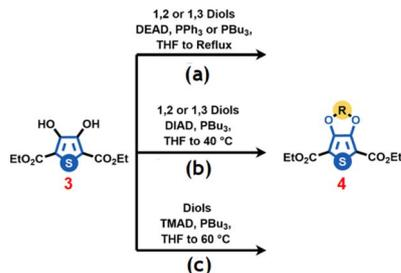
Scheme 3 O-alkylation of 3,4-dialkoxythiophenes based on the Mitsunobu reaction using (a) diethyl azodicarboxylate (DEAD), (b) dialkylazodicarboxylate (DIAD) and (c) tetramethylazodicarboxamide (TMAD) as dehydrogenating agents.
