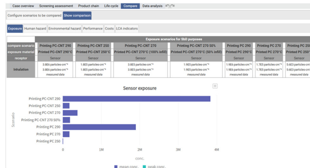
Fig. 5 Comparison of release results obtained by the air monitoring campaign performed before ( i.e. , PC-SWCNT.290) and after SbD implementations (PC-SWCNT.250, PC-SWCNT.270, and PC-SWCNT.270-50%) as well as during the production of the PC without SWCNTs ( i.e. , PC-290, PC-270, and PC-250).
