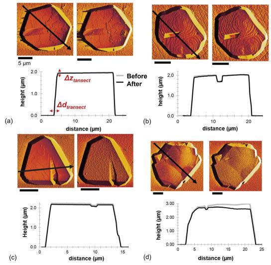
Fig. 2 AFM deflection imaging showing changes in hematite particle microtopography ex situ, following reaction with (a) KCI, (b) Fe(II), (c) oxalate, and (d) Fe(ii)-oxalate. Transectional analyses from correlative Z-sensor imaging highlights changes in particle heights and diameters across select regions (marked with black arrows). Scale bar in images represents 5  $\mu m$ .
