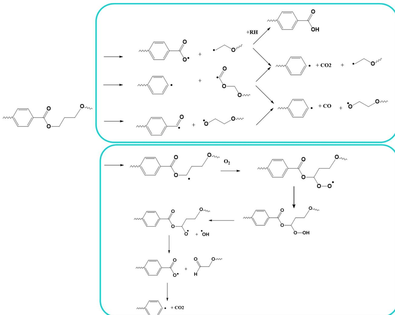
Fig. 18 Top: Reported overall mechanisms for photo-oxidative degradation. Bottom: specific mechanism for vacuum photolysis and photo-oxidation. Reactions based on the work by Day *et al.*<sup>133</sup>
