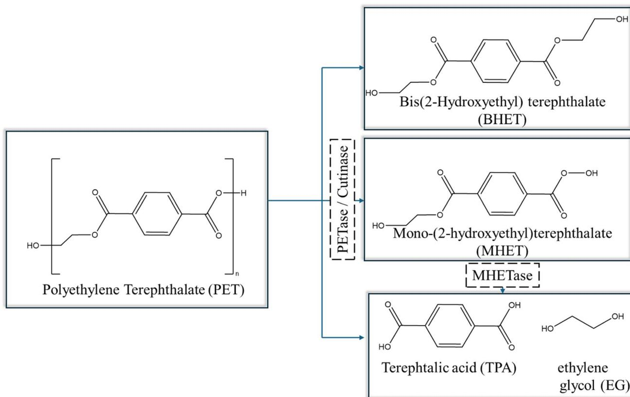
Fig. 22 Overall reactions for PET degradation catalysed by PETase or cutinase based on the work by Khairul Anuar.<sup>147</sup>
