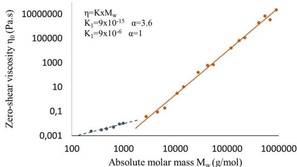
Fig. 34 Zero-shear viscosity as a function of mass (weight) average molar mass for linear polyethylenes, considering a wide range of molar masses and dispersity. Data to construct the figure from Münstedt.<sup>192</sup>
