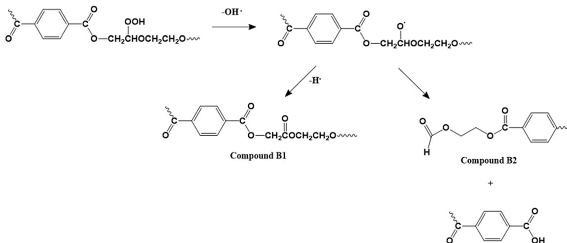
Fig. 16 Thermo-oxidative degradation mechanism with a DEG comonomer unit based on the work by Romão *et al.*<sup>125</sup>
