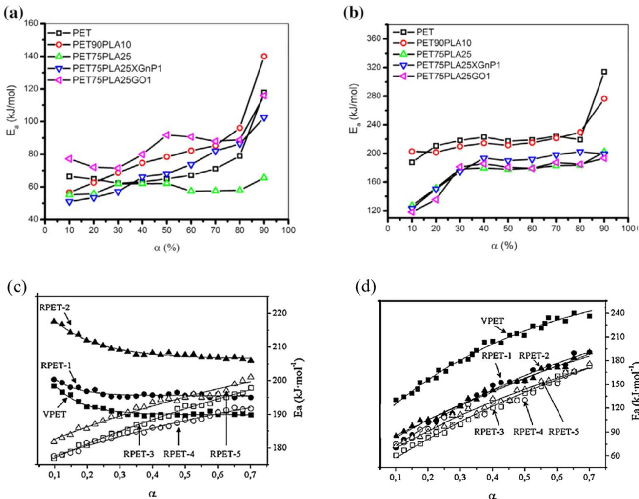
Fig. 25 TGA results for blends with PET (top row a and b) and comparison of virgin and recycled PET (bottom row c and d).<sup>103,159</sup> Reproduced with permission from the publishers Elsevier and John Wiley & Sons; where  $\alpha$  is conversion (either in % (top) or as fraction (bottom)).
