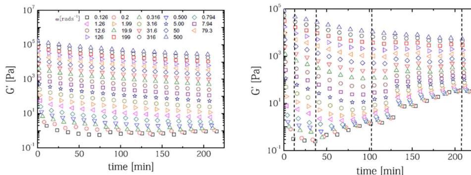
Fig. 37 Time-resolved mechanical spectroscopy (TRMS) of the storage modulus,  $G'$ , at different frequencies ( $\omega$  values): left 265 °C and right 288 °C. Measurement performed in the air.<sup>202</sup> Reproduced with permission from the publisher Springer Nature.
