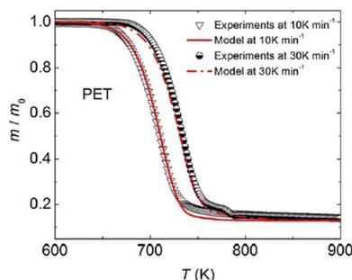
Fig. 24 Example of application of TGA to obtain lumped kinetic parameters, typically for chemical recycling (or very strong degradation) of polyesters.<sup>157</sup> Reproduced with permission from the publisher Elsevier.
