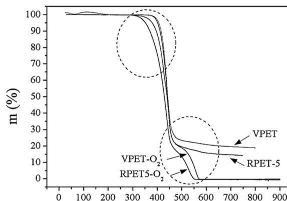
Fig. 40 TGA analysis of virgin PET (VPET) and PET reprocessed 5 times (RPET-5). Two cases are considered: an inert atmosphere and under oxygen.<sup>103</sup> Reproduced with permission from Elsevier.
