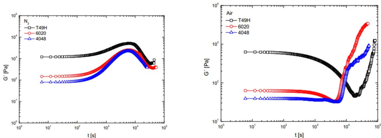
Fig. 31 Storage modulus ( $G'$ ) measured as a function of time in the presence of nitrogen (left) and air (right) of 3 different PET grades: PET T49H (black), 6020 (red) and 4048 (blue). Temperature of 280 °C, frequency of 10 rad s<sup>-1</sup> and deformation of 10%.<sup>188</sup> Reproduced with permission from the publisher, AIP Publishing.
