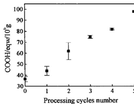
Fig. 10 Variation in the carboxylic end group concentration as a function of the number of processing cycles for PET thermal degradation.<sup>105</sup> Reproduced with permission from the publisher John Wiley & Sons.
