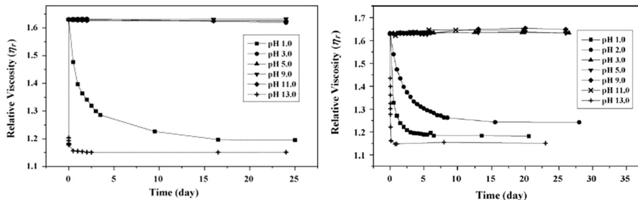
Fig. 28 Relative viscosity of solution with PLA (left) and PPC (right; 0.5 wt% polymer) at different pH.<sup>164</sup> Reproduced with permissions from the publisher Elsevier.
