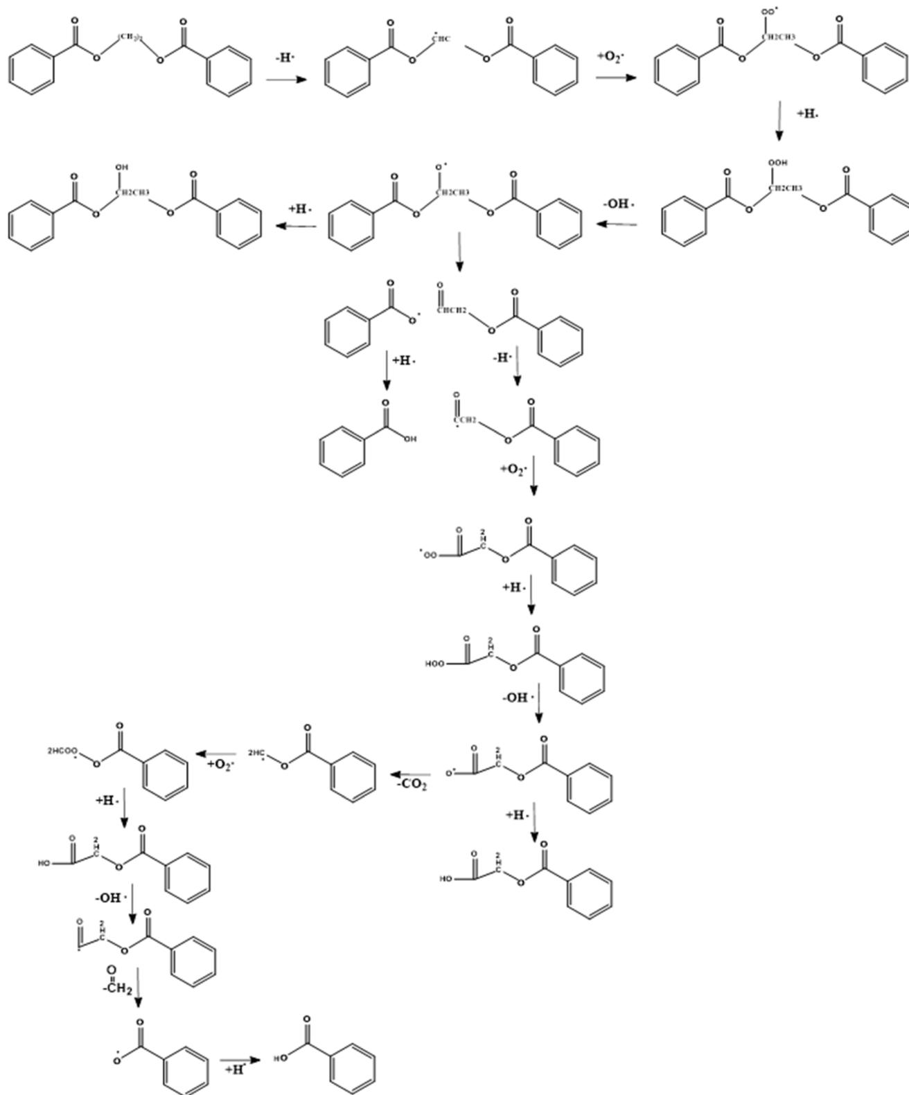
Fig. 13 First mechanism of thermo-oxidative degradation of ethylene dibenzoate (EDB) being a model compound for PET. This mechanism is based on the work by Botelho *et al.*<sup>118</sup>
