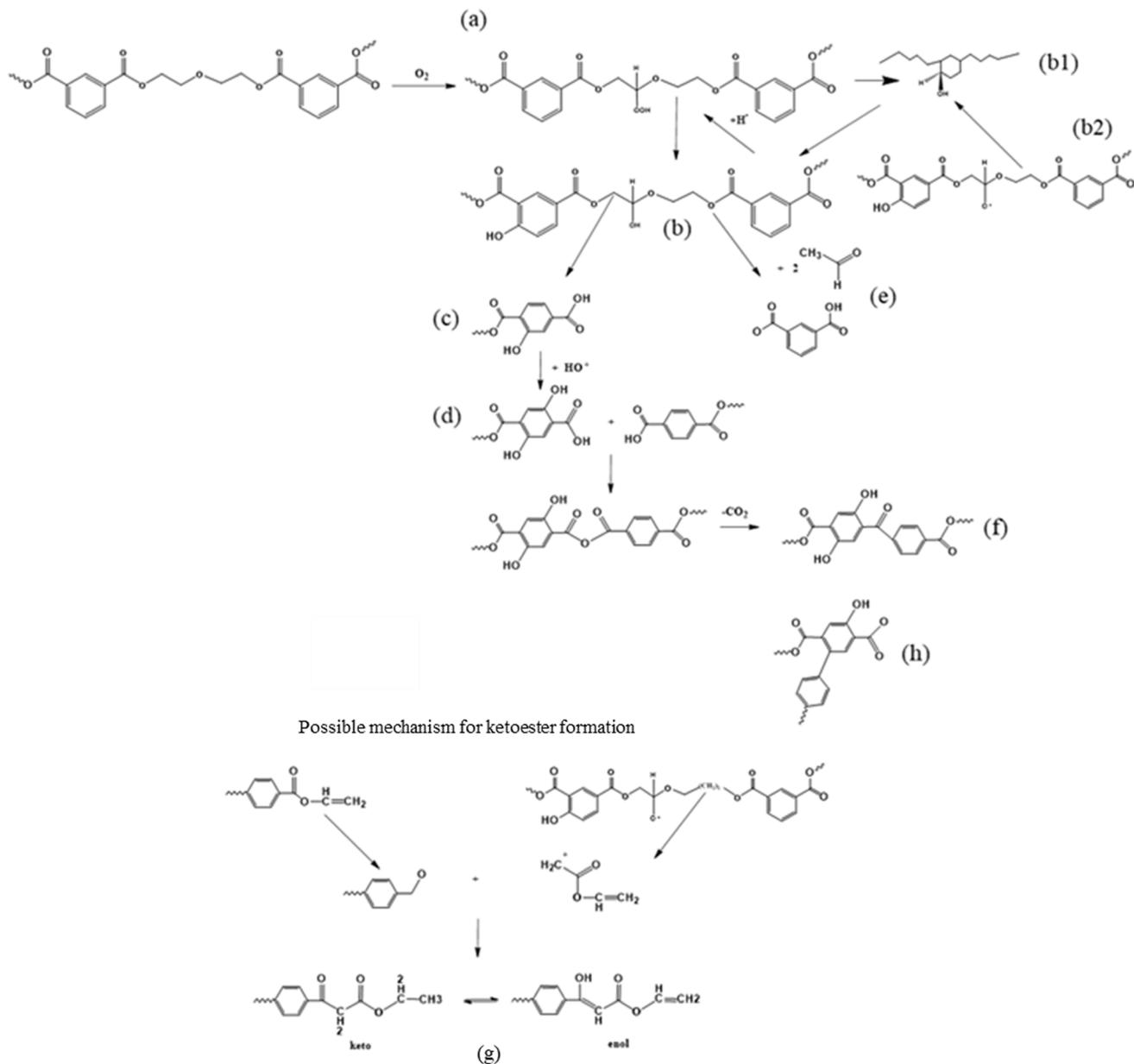
Fig. 14 Second mechanism of thermo-oxidative degradation of PET. This mechanism is based on the work by Ciolacu *et al.*<sup>121</sup>
