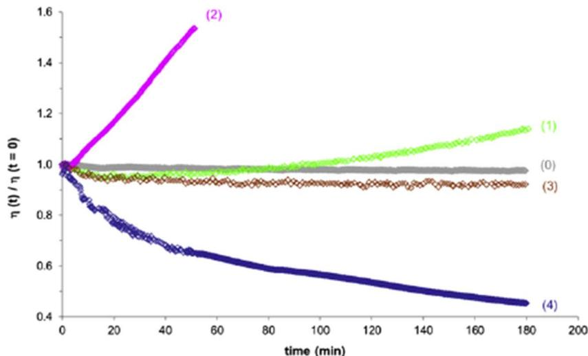
Fig. 35 PET zero-shear or Newtonian viscosity as a function of time (divided by the initial value) at oxygen partial pressures of 0%, 0.6%, 1%, 9%, and 21% (at 280 °C).<sup>160</sup> Reproduced with permission from the publisher Elsevier.
