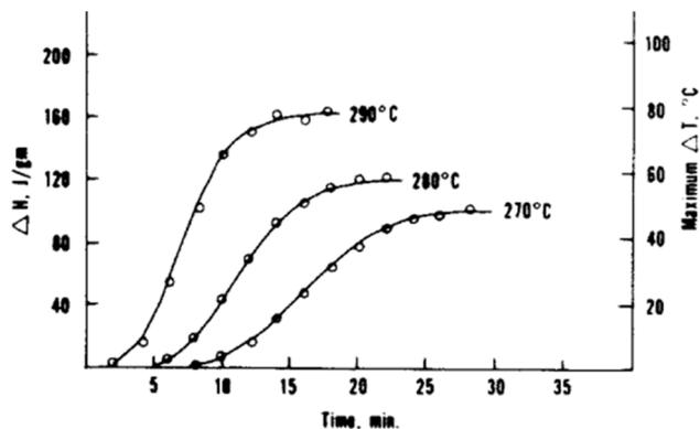
Fig. 43 DSC enthalpy data regarding the exothermic peak of PET. The measurements were conducted in isothermal mode for a certain time. The curves are parametric to the melting temperature.<sup>120</sup> Reproduced with permission from the publisher John Wiley and Sons.
