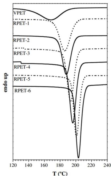
Fig. 42 DSC curves of PET during the first cooling cycle.<sup>209</sup> Reproduced with permission from the publisher Elsevier.
