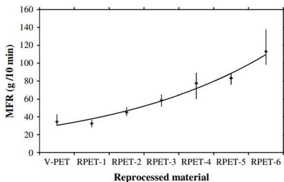
Fig. 39 Evolution of melt-mass flow rate (MFR) through reprocessing simulation.<sup>209</sup> Reproduced with permission from the publisher Elsevier.
