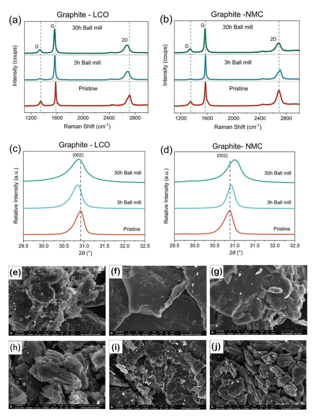
Fig. 2 Comparison of the impact of ball milling on PRG, Raman spectra of (a) PRG-LCO and (b) PRG-NMC, (c) XRD patterns in selected  $2\theta$  regions highlighting the (002) reflection of (d) PRG-LCO and (e) PRG-NMC, microstructures of (e) PRG-LCO, (f) PRG-LCO-3h, and (g) PRG-LCO-3h, and microstructures of (h) PRG-NMC, (i) PRG-NMC-3h, and (j) PRG-NMC-30h.
