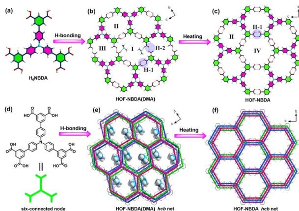
Fig. 9 (a) The structure of  $\text{H}_6\text{NBDA}$ ; (b and c) representation of the reorganization of H-bond dimers upon heating; (d) scheme of  $\text{H}_6\text{NBDA}$  and the six-connected node; (e and f) the transformation of layered frameworks before and after heating.<sup>67</sup>
