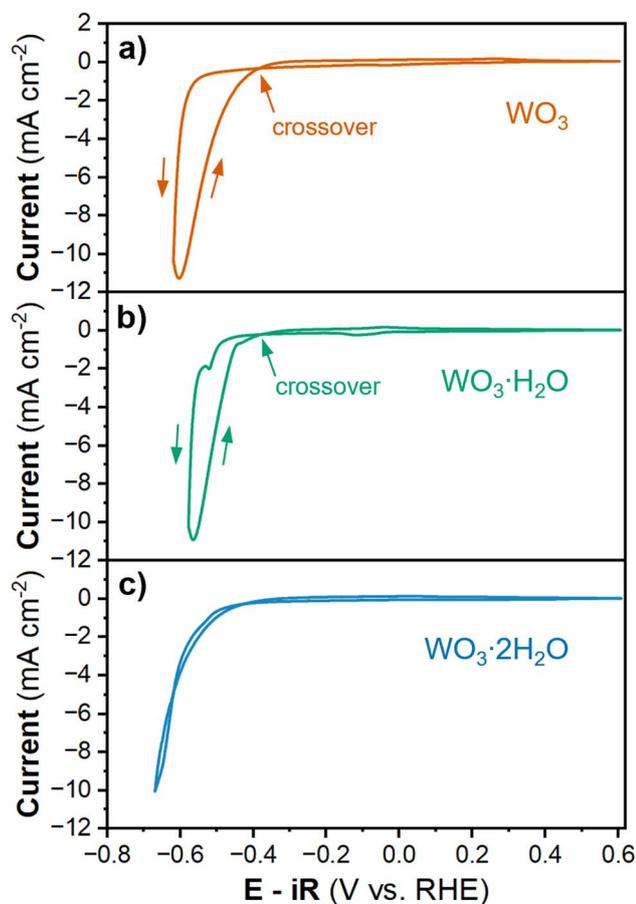
Fig. 3 Cyclic voltammograms of (a)  $\text{WO}_3$ , (b)  $\text{WO}_3 \cdot \text{H}_2\text{O}$ , and (c)  $\text{WO}_3 \cdot 2\text{H}_2\text{O}$  where the cathodic potential limit was set to the potential where current reaches  $10 \text{ mA cm}^{-2}$ . The scan rate was  $10 \text{ mV s}^{-1}$  and rotation rate was 1600 rpm.
