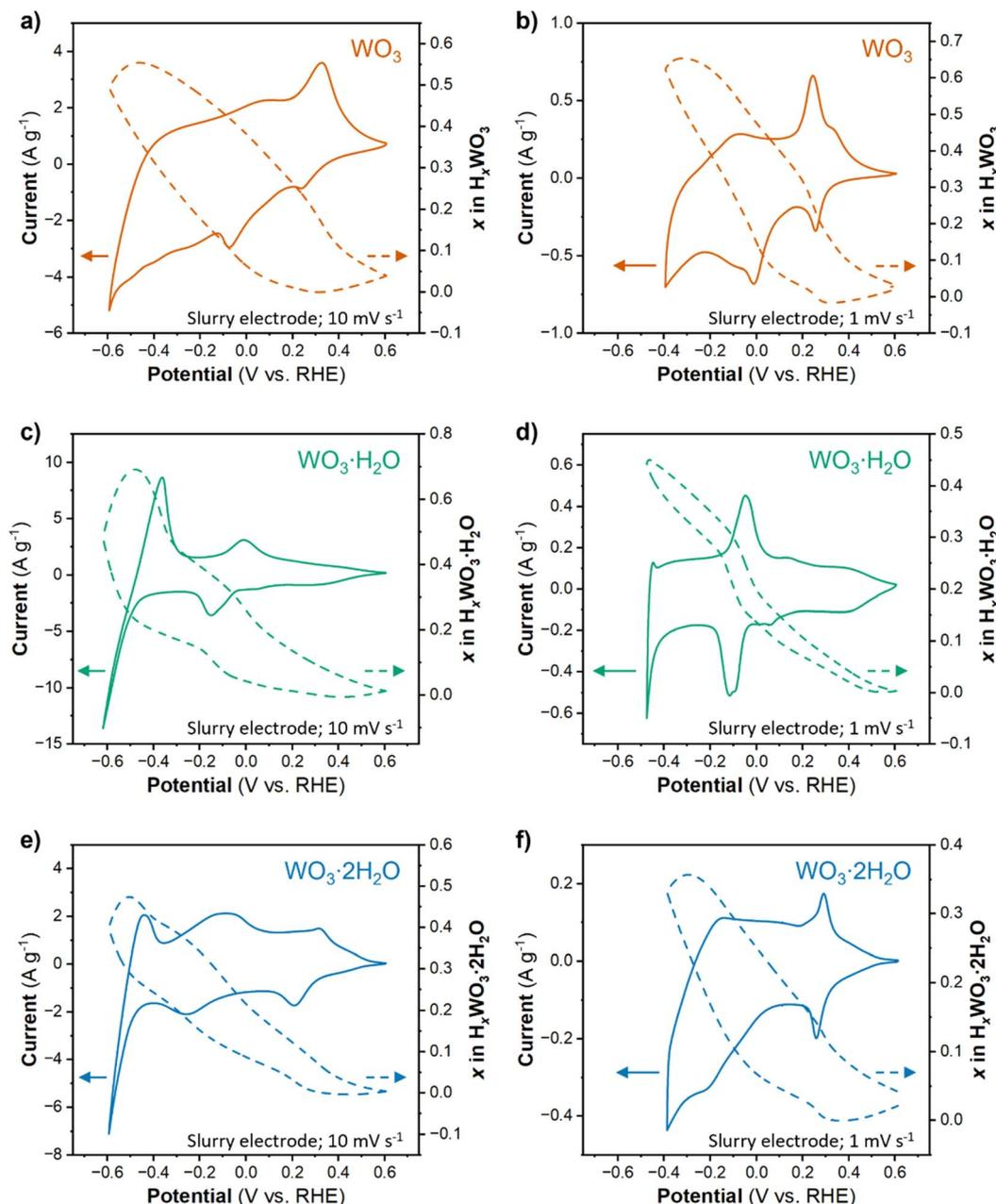
Fig. 5 CVs and proton composition as a function of potential for slurry electrodes of (a and b)  $\text{WO}_3$ , (c and d)  $\text{WO}_3 \cdot \text{H}_2\text{O}$ , and (e and f)  $\text{WO}_3 \cdot 2\text{H}_2\text{O}$  at  $10 \text{ mV s}^{-1}$  (a, c and e) and  $1 \text{ mV s}^{-1}$  (b, d and f) in  $0.5 \text{ M H}_2\text{SO}_4$ . Solid lines indicate the current, and dashed lines indicate the proton composition as a function of potential.
