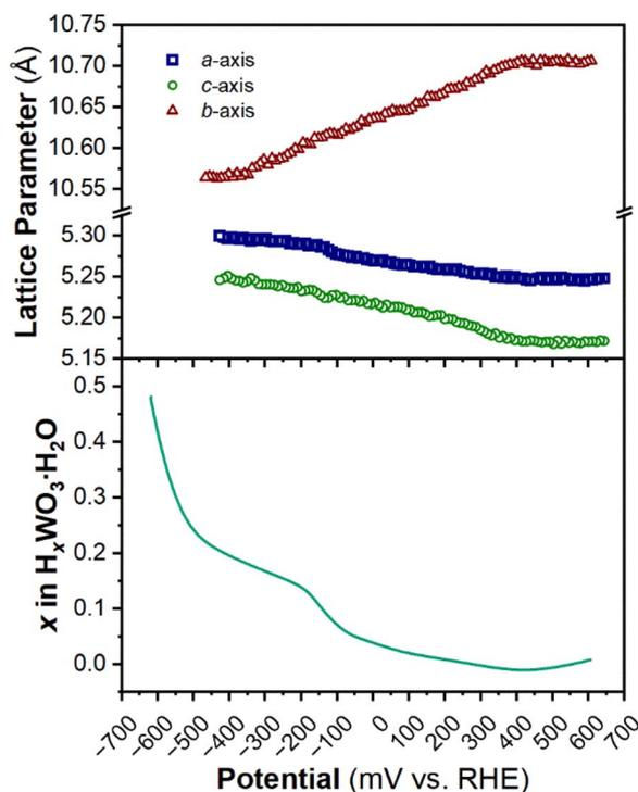
Fig. 9 Trend of lattice parameters (from Pawley refinements of the operando XRD) and proton composition in  $\text{H}_x\text{WO}_3 \cdot \text{H}_2\text{O}$  (from Fig. 5c) as a function of potential during the cathodic cyclic voltammetry scan in  $0.5 \text{ M H}_2\text{SO}_4$  at  $10 \text{ mV s}^{-1}$ .
