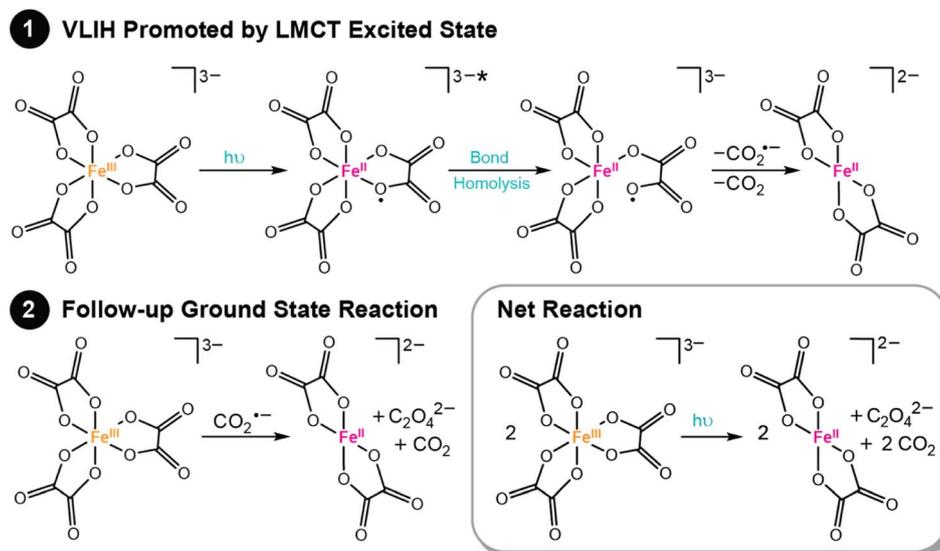
Fig. 3 VLIH mechanism of ferrioxalate to form ferrous oxalate. Further decomposition of the  $\text{C}_2\text{O}_4^{\bullet-}$  with a second equivalence of ferric oxalate yields an additional equivalence of ferrous oxalate and two equivalents of  $\text{CO}_2$ .
