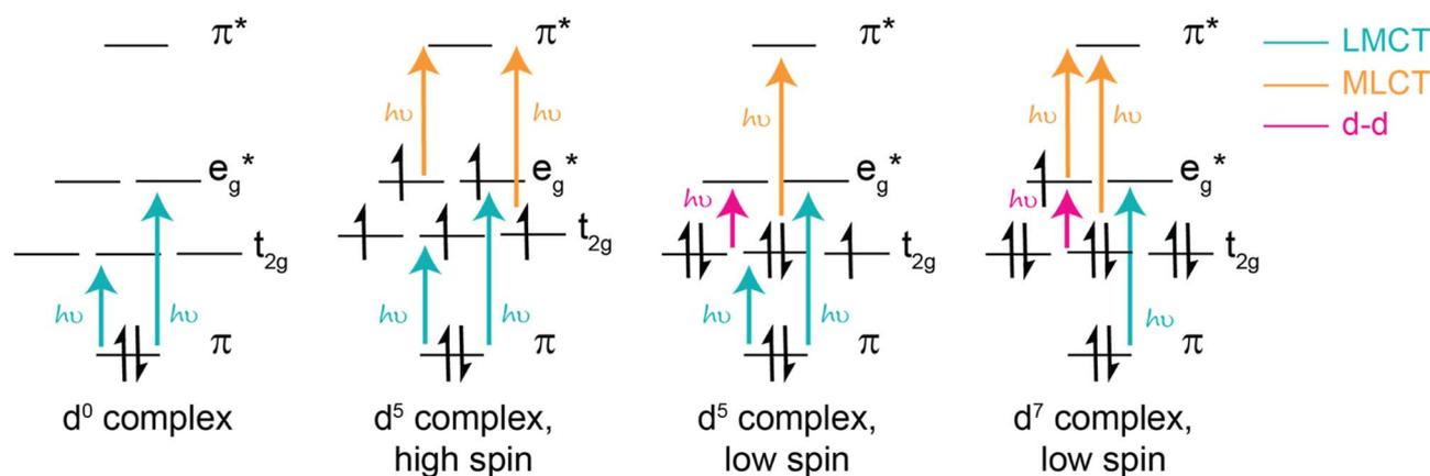
Fig. 2 Examples of accessible excited states from  $d^0$ ,  $d^5$ , and  $d^7$  complexes, which most commonly exhibit LMCT. In addition, it is important to note the bonding character of the metal-based  $t_{2g}$  orbitals depends on the nature of the coordinating ligands. Strong  $\pi$  donors facilitate antibonding  $t_{2g}$  orbitals,  $\sigma$  donors promote non-bonding  $t_{2g}$  orbitals, and  $\pi$  acceptors facilitate bonding  $t_{2g}$  orbitals.
